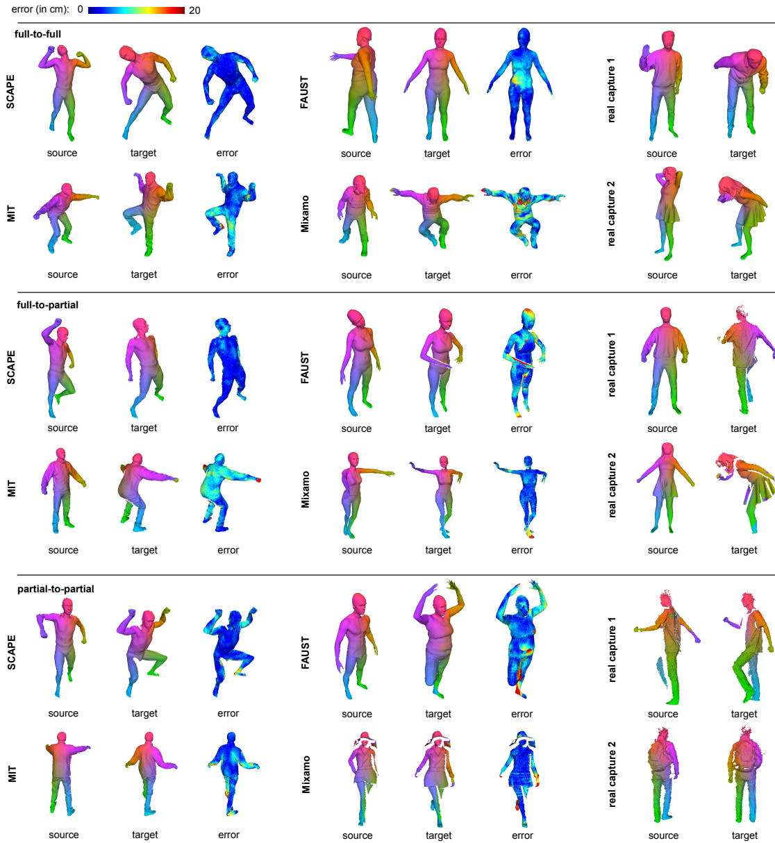
Figure 3.7: Deep learning-based correspondence computation can handle full-to-full, partial-to-full, and partial-to-partial matchings between full 3D models and partial scans generated from a single depth map. This method is evaluated on various real and synthetic datasets.
